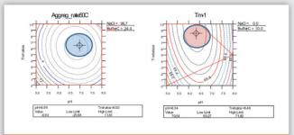
Figure 5. The areas identified for minimal aggregation rates and maximum Tm-1 values. Shaded areas shows optimal design spaces for minimal aggregation rates and maximum Tm-1 for each response.
