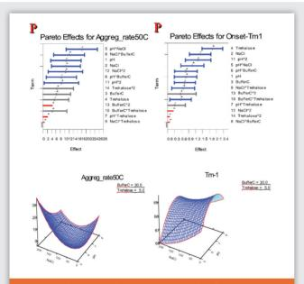
Figure 4. The top panel shows the Pareto plots for aggregation rates and Tm-1. The bottom panel shows the 3D response surface plots for NaCl and pH for aggregation rates and Tm-1.
